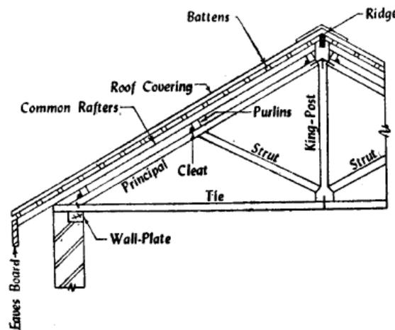
Fig 13.8 King post truss roof
