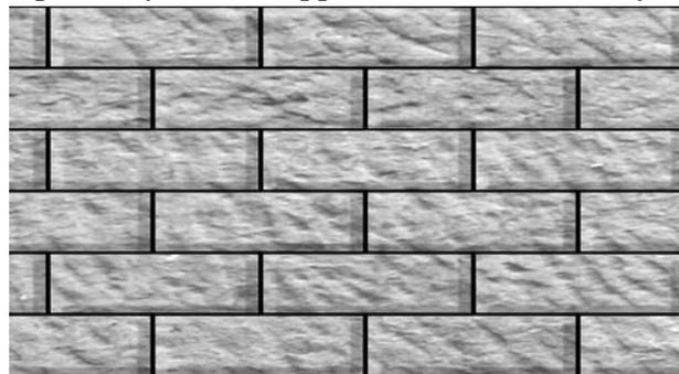
2. **Ashlar rough-tooled masonry:** In this type of ashlar masonry, the beds and sides, are finely chisel-dressed. But the face is made rough by means of tools. A strip about 25mm wide and made by means of a chisel is provided around the perimeter of every stone exposed for view. The thickness of the mortar joints does not exceed 6mm. This type of work is also known as the bastard ashlar.
