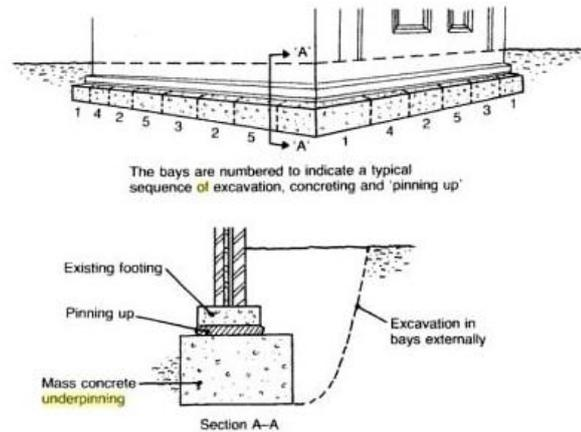
**Fig.1: Mass Concrete Underpinning**
