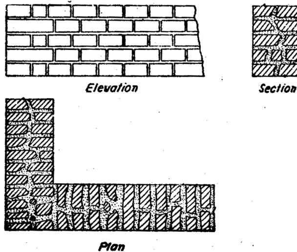
**Polygonal rubble masonry:** In this type of masonry the stones are roughly dressed to an irregular polygonal shape. The stones should be so arranged as to avoid long vertical joints in face work and to break joints as much as possible. Small stone chips should not be used to support the stones on the facing as shown in fig
