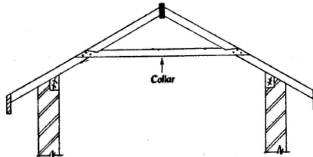
Fig 13.6 Collar beam roof
