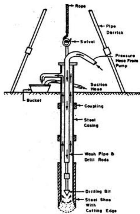
(c) Rotary boring: is a very fast method of advancing hole in both rocks and soils. A drill bit, fixed to the lower end of the drill rods, is rotated by a suitable chuck and is always kept in firm contact with the bottom of the hole. A drilling mud usually a water solution of bentonite with or without other admixtures is continuously forced down to the hollow drill rods. The mud returning upwards brings the cuttings to the surface.
