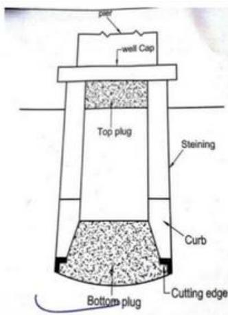
**Open caissons** are small cofferdams that are placed and then pumped dry and filled with concrete. These are generally used in the formation of a pier.
