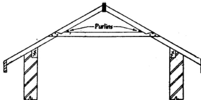
Fig 13.7 Double or Purlin roof
