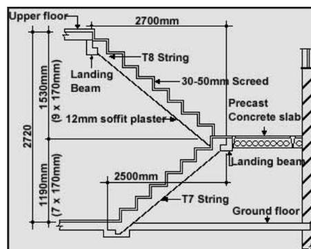
(iii) **Open-Newel stairs:** It consists of two or more straight flights arranged in such a manner that a clear space called a “well” occurs between the backward and forward flights.
