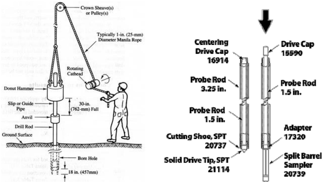
(iii) **Sub-surface sounding (SPT Test):** In this method, the resistance of the soil with depth is measured by means of a tool known as pentrometer under static or dynamic loading.
