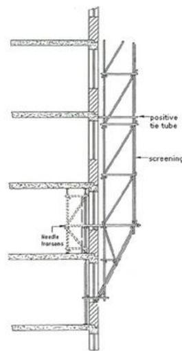
The American National Standards Institute describes **scaffolding** as “a temporary elevated or suspended work unit and its supporting structure used for supporting worker(s) or materials, or both,” while the same agency describes **shoring** as “The vertical supporting members in a formwork system.”
