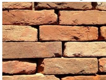
c. **Third class bricks:** These bricks are ground moulded and they are burnt in clamps. These bricks are not hard and they have rough surfaces with irregular and distorted edges. These bricks give a dull sound when struck together. They are used for unimportant and temporary structures and in places where rainfall is not heavy.
