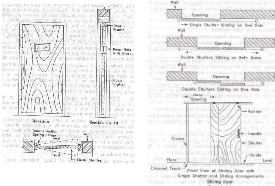
Swing doors are generally provided in passage of public buildings. The doors may have single or two shutters. The shutters are fixed with special hinges known as double action spring hinges which hold the shutter in closed position when not in use.
