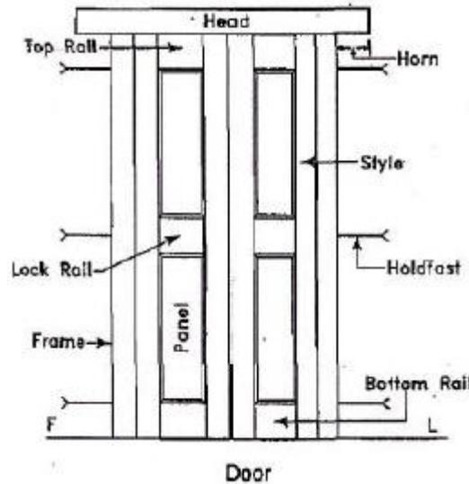
Panel: The portion inside the shutter frame work in termed as panel.
