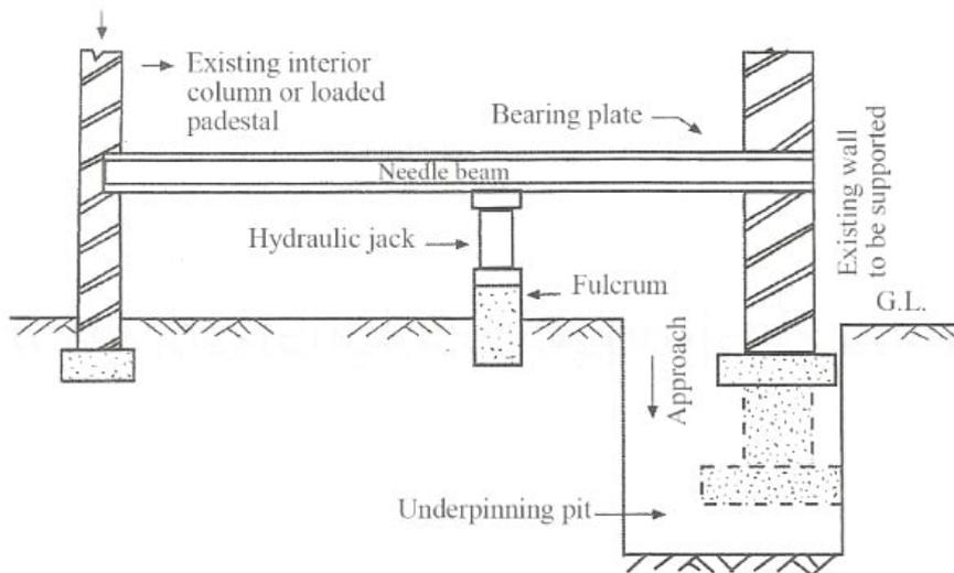
**Fig.2: Cantilever Needle Beam Underpinning Method**
