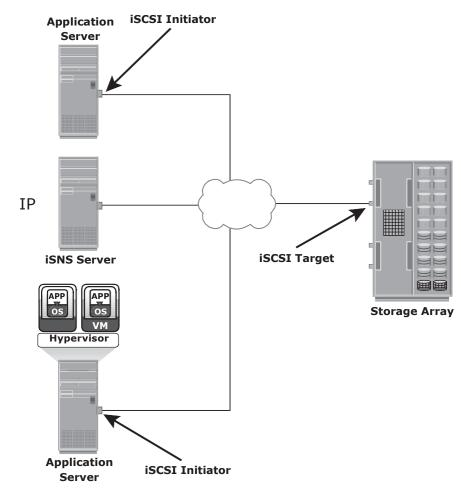
Figure 6-6: Discovery using iSNS
