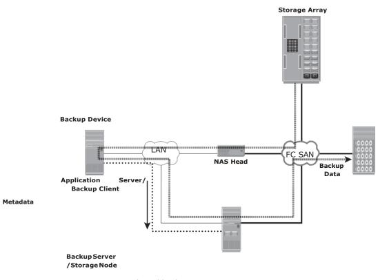
Figure 10-11: Server-based backup in a NAS environment
