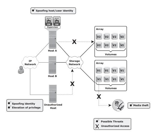
Figure 14-2: Security threats in an application access domain
