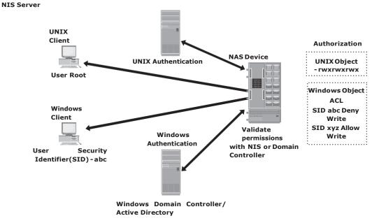
Figure 14-7: Securing user access in a NAS environment
