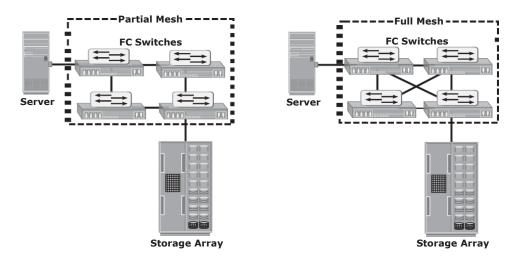
Figure 5-20: Partial mesh and full mesh topologies
