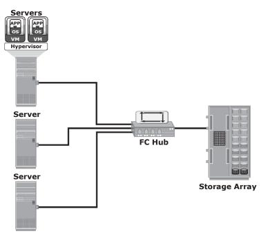
Figure 5-7: Fibre Channel Arbitrated Loop
