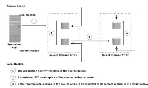
Figure 12-9: Disk-buffered remote replication
