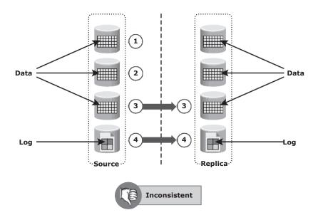
Figure 11-4: Inconsistent database replica
