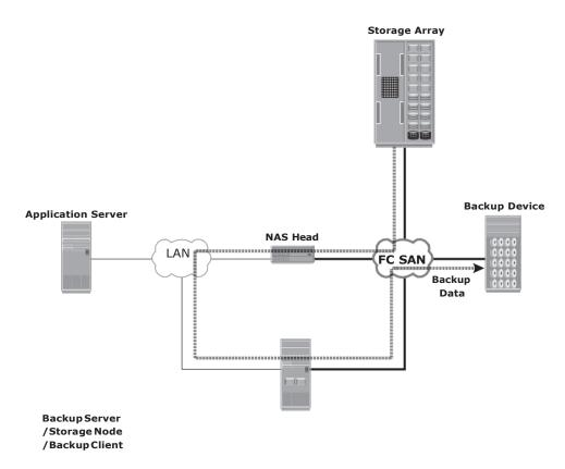
Figure 10-12: Serverless backup in a NAS environment
