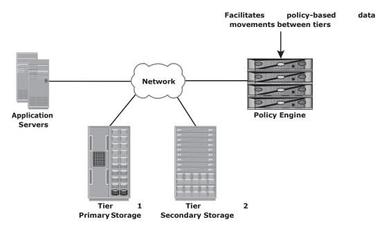
Figure 15-14: Implementation of inter-array storage tiering
