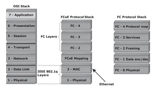
Figure 6-17: FCoE frame mapping
