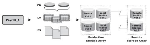
Figure 15-10: Correlation of capacity configured for an application
