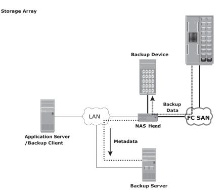
Figure 10-13: NDMP 2-way in a NAS environment
