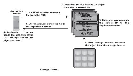
Figure 8-6: Object retrieval from an OSD system
