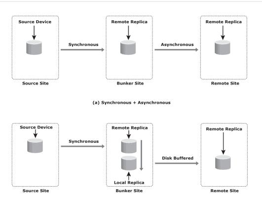
(b) Synchronous + Disk Buffered
