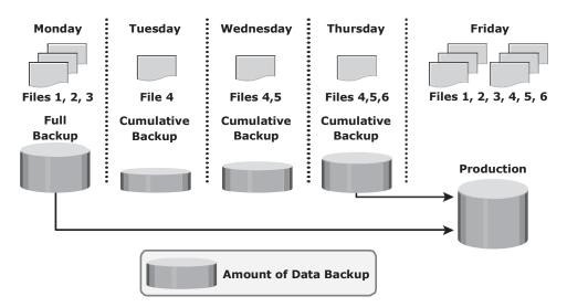
Figure 10-3: Restoring a cumulative backup
