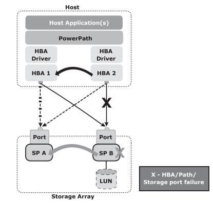
Figure 9-11: Path failover with PowerPath for an active-passive array
