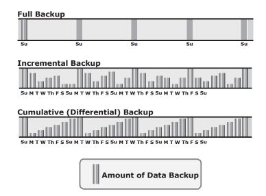
Figure 10-1: Backup granularity levels
