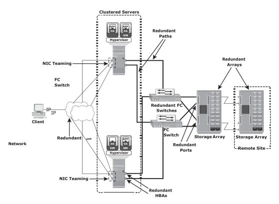
Figure 9-6: Resolving single points of failure
