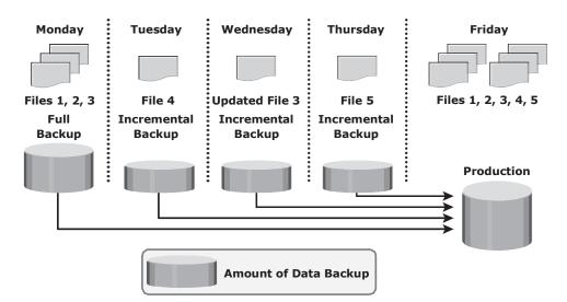
Figure 10-2: Restoring from an incremental backup
