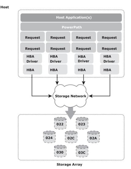
Figure 9-8: I/O with PowerPath
