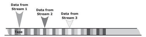
Figure 10-16: Multiple streams on tape media
