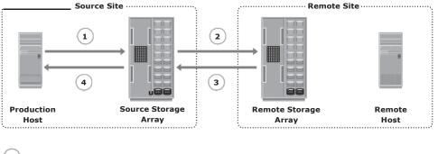
f 1 ) Write from the production host is received by the source storage array.
