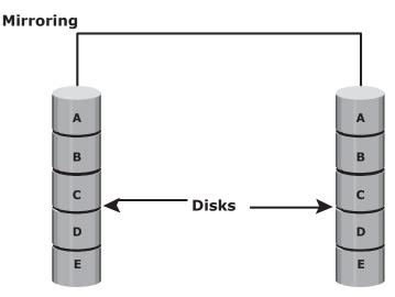
Figure 3-3: Mirrored disks in an array
