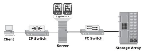
Figure 9-5: Single point of failure
