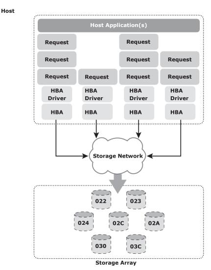
Figure 9-7: I/O without PowerPath
