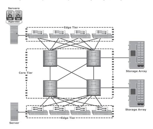
Figure 5-23: Compound core-edge topology
