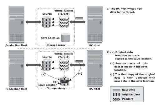
Figure 11-13: Pointer-based virtual replication — write to target
