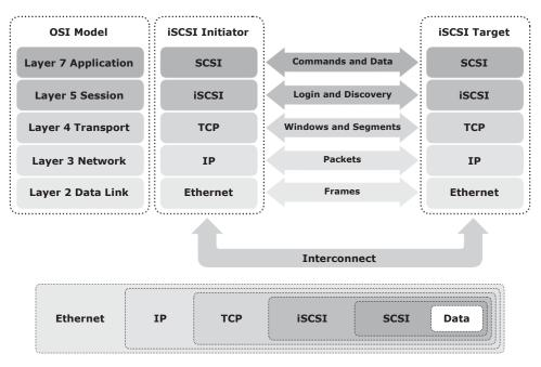
Figure 6-3: iSCSI protocol stack
