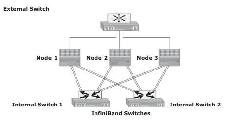
Figure 7-7: Scale-out NAS with dual internal and single external networks
