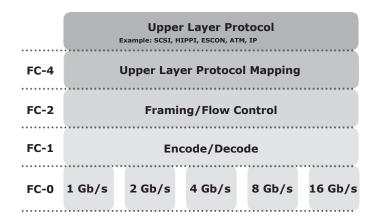
Figure 5-12: Fibre Channel protocol stack
