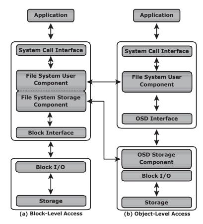
Figure 8-3: Block-level access versus object-level access
