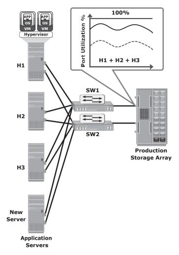
Figure 15-4: Monitoring array port utilization
