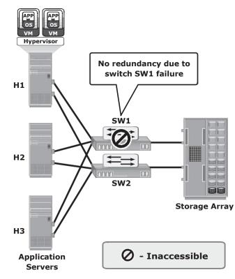
Figure 15-1: Switch failure in a storage infrastructure
