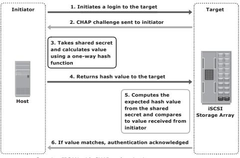
Figure 14-10: Securing IPSAN with CHAP authentication
