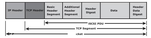
Figure 6-4: iSCSI PDU encapsulated in an IP packet
