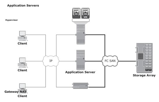
Figure 7-6: Gateway NAS connectivity
