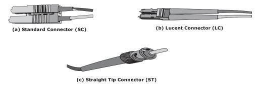
Figure 5-5: SC, LC, and ST connectors
