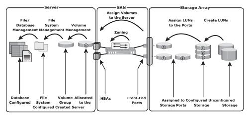
Figure 15-7: Storage allocation tasks
