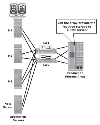
Figure 15-2: Monitoring storage array capacity
