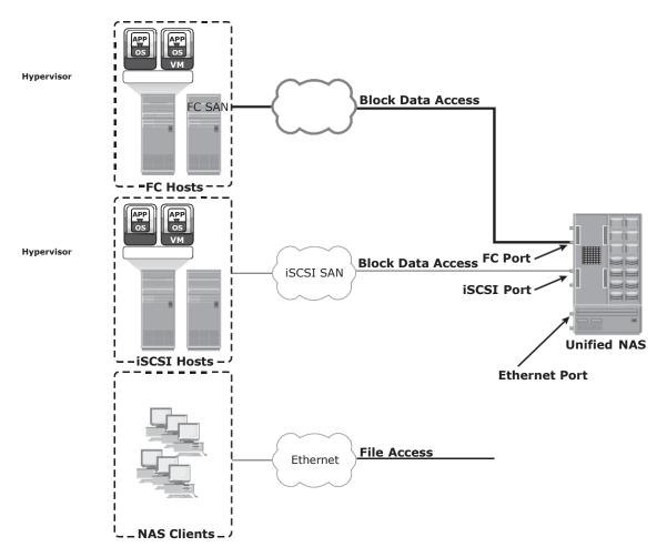
Figure 7-5: Unified NAS connectivity
