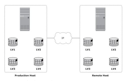
Figure 12-5: LVM-based remote replication
