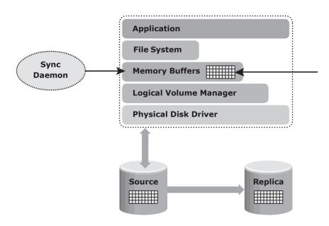
Figure 11-1: Flushing the file system buffer
