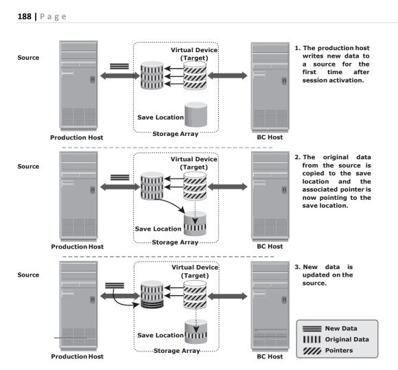
Figure 11-12: Pointer-based virtual replication — write to source
