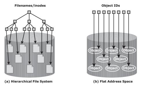
Figure 8-1: Hierarchical file system versus flat address space
