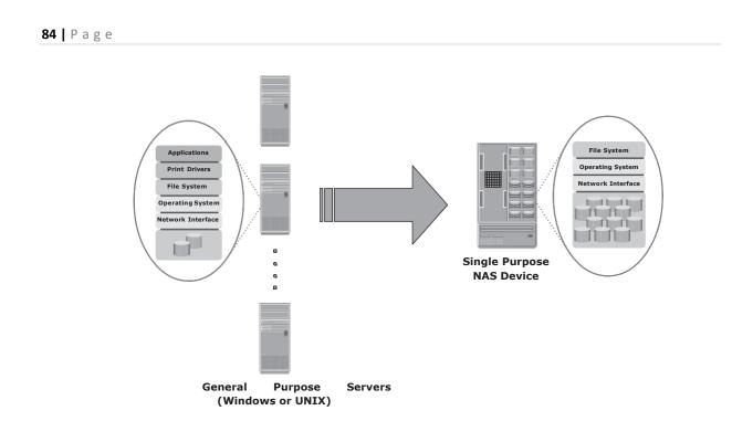
Figure 7-1: General purpose server versus NAS device
