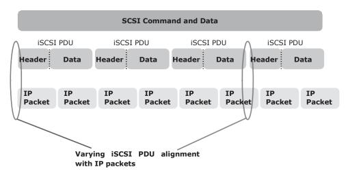
Figure 6-5: Alignment of iSCSI PDUs with IP packets
