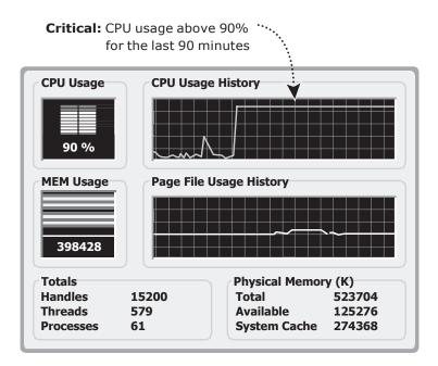
Figure 15-5: Monitoring the CPU and memory usage of a server
