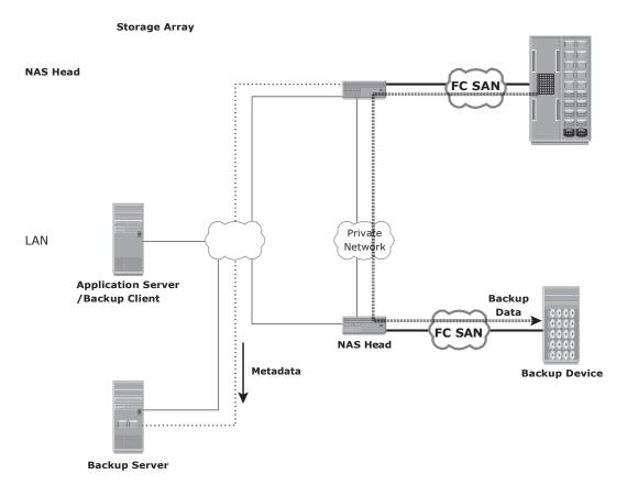
Figure 10-14: NDMP 3-way in a NAS environment
