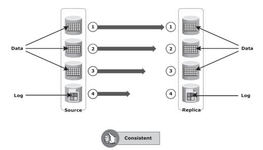
Figure 11-3: Dependent write consistency on replica
