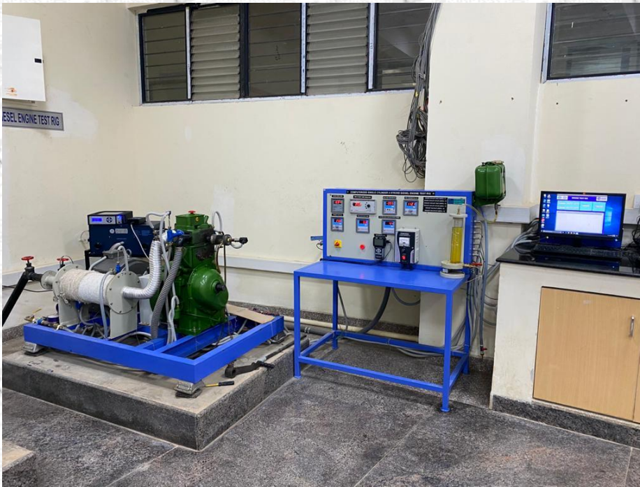
Computerized engine test rig
