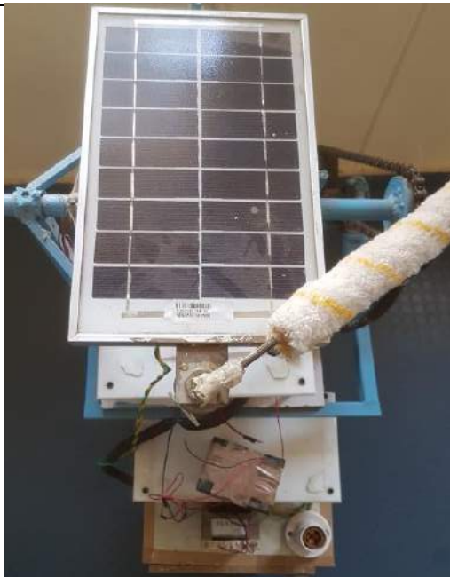
Solar PV panel with built in cleaning assembly
