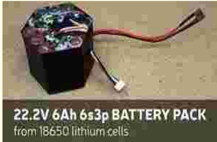
The recommended way to build the packs is by using the 18650 battery holders which are also available at low cost.
